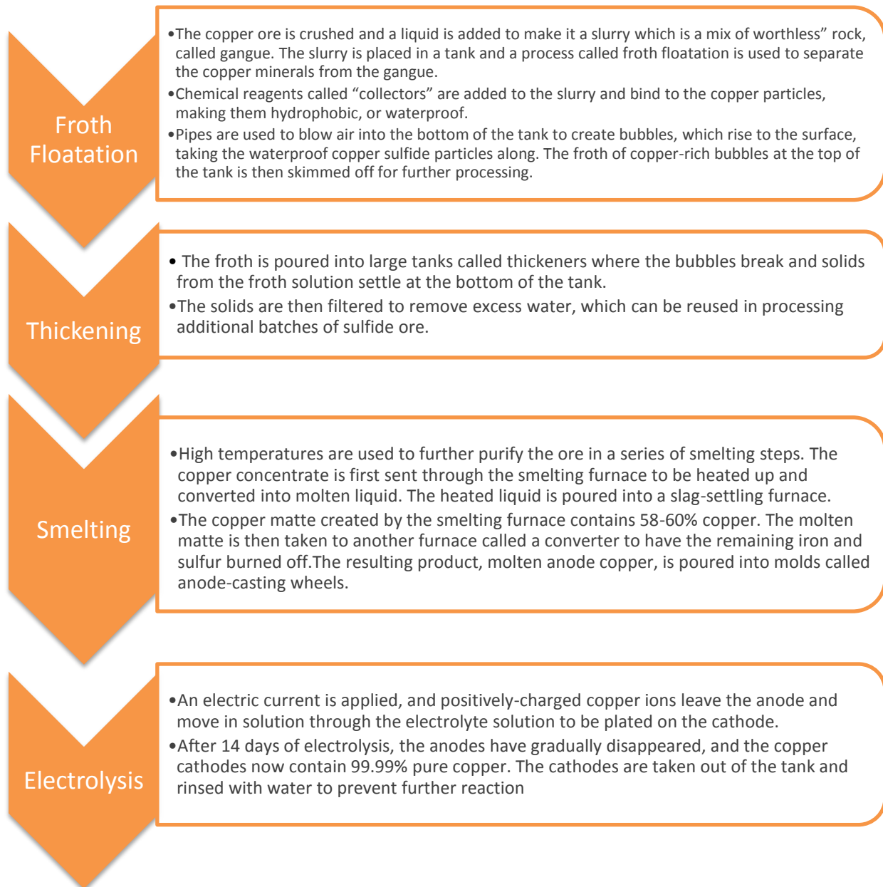
Chart : Process of copper refining through Pyrometallurgy
